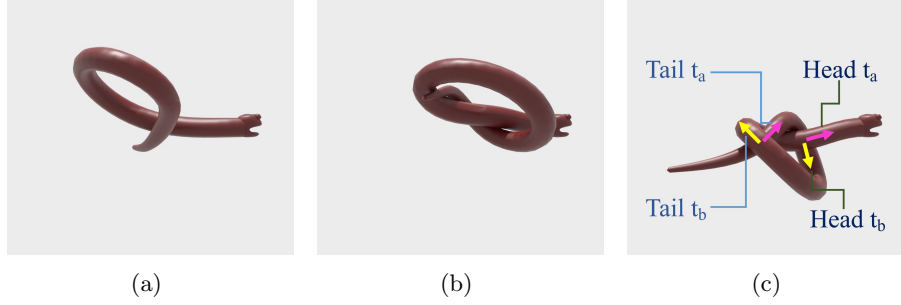
Fig. 4: Simulation of knot formulation. We closely follow each kinematic steps of hagfish behavior: (a) body crossover, (b) tail wrap, and (c) tail insertion. The labeled tangents in (c) are for the thigmotaxis constraints used in knot sliding.
