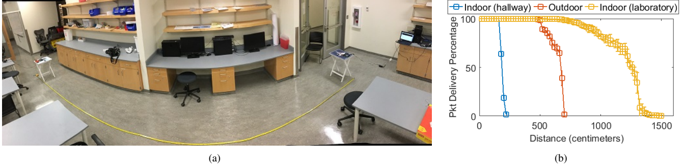
Fig. 3. (a) Experimental location in laboratory, and (b) Packet delivery percentage with distance in different environments.
