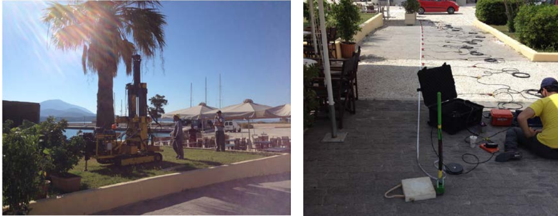
Figure 6. (a) DPT performed in a planter box at the Lixouri Port and (b) MASW performed next to the planter box.
