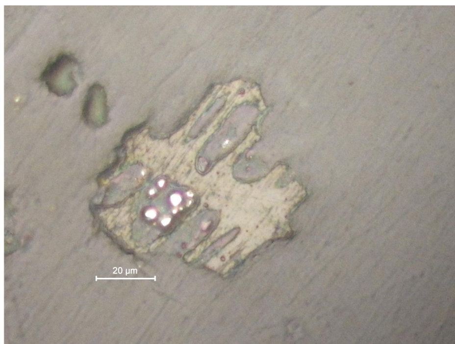
Figure S-5 Representative images of polished charcoal fragments from WL and RF. Note smooth, well-preserved cell walls present in the samples. Bright areas are post-depositional pyrite.
