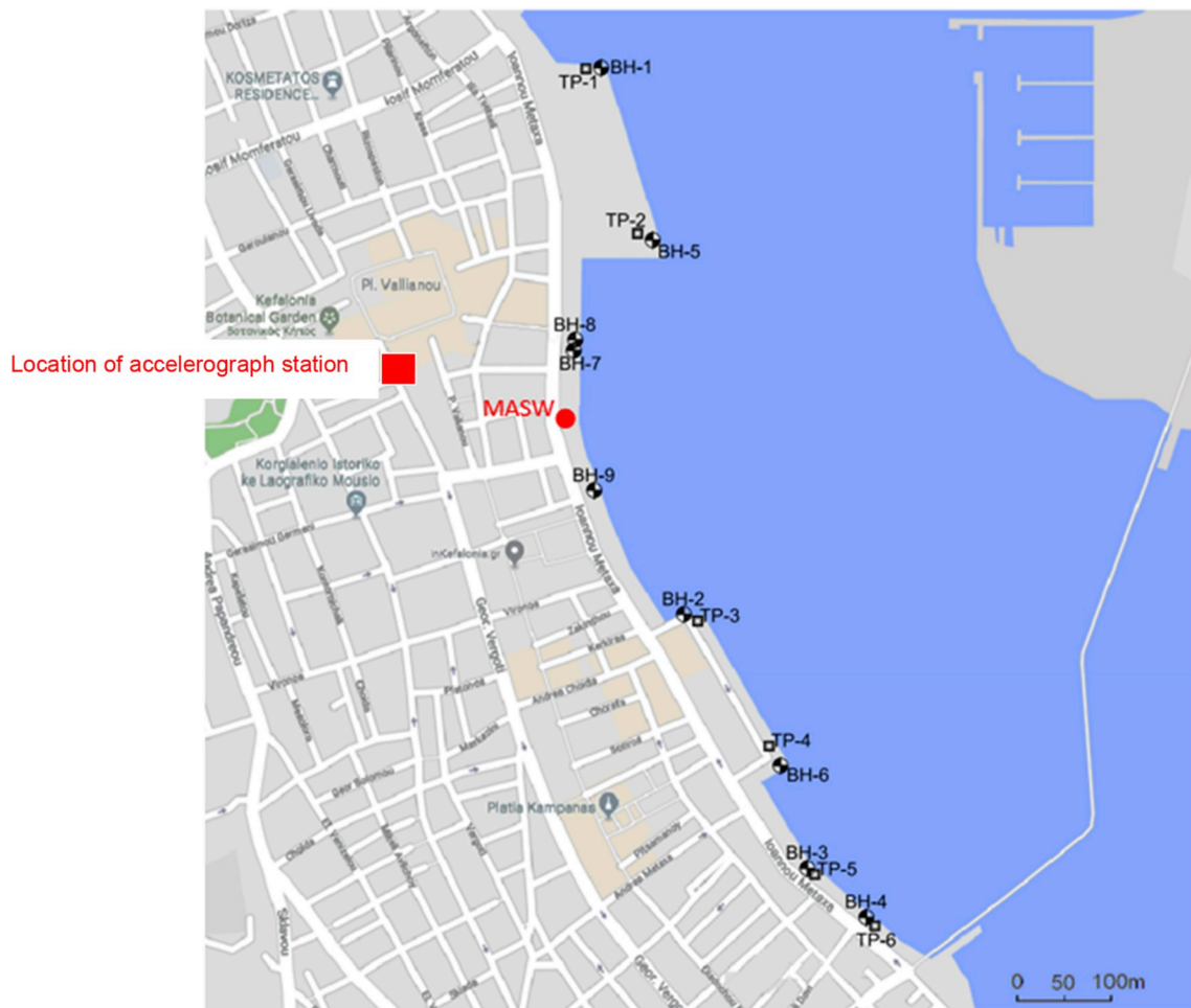
Fig. 12. Location of boreholes, test pits, MASW measurements and acceleration station in the Argostoli Port area.
