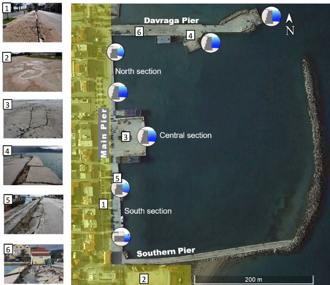
Fig. 2. Satellite image of the Lixouri Port area (liquefied area indicated by yellow shading and location of photos indicated by numbered white squares). (For interpretation of the references to color in this figure legend, the reader is referred to the Web version of this article.)
