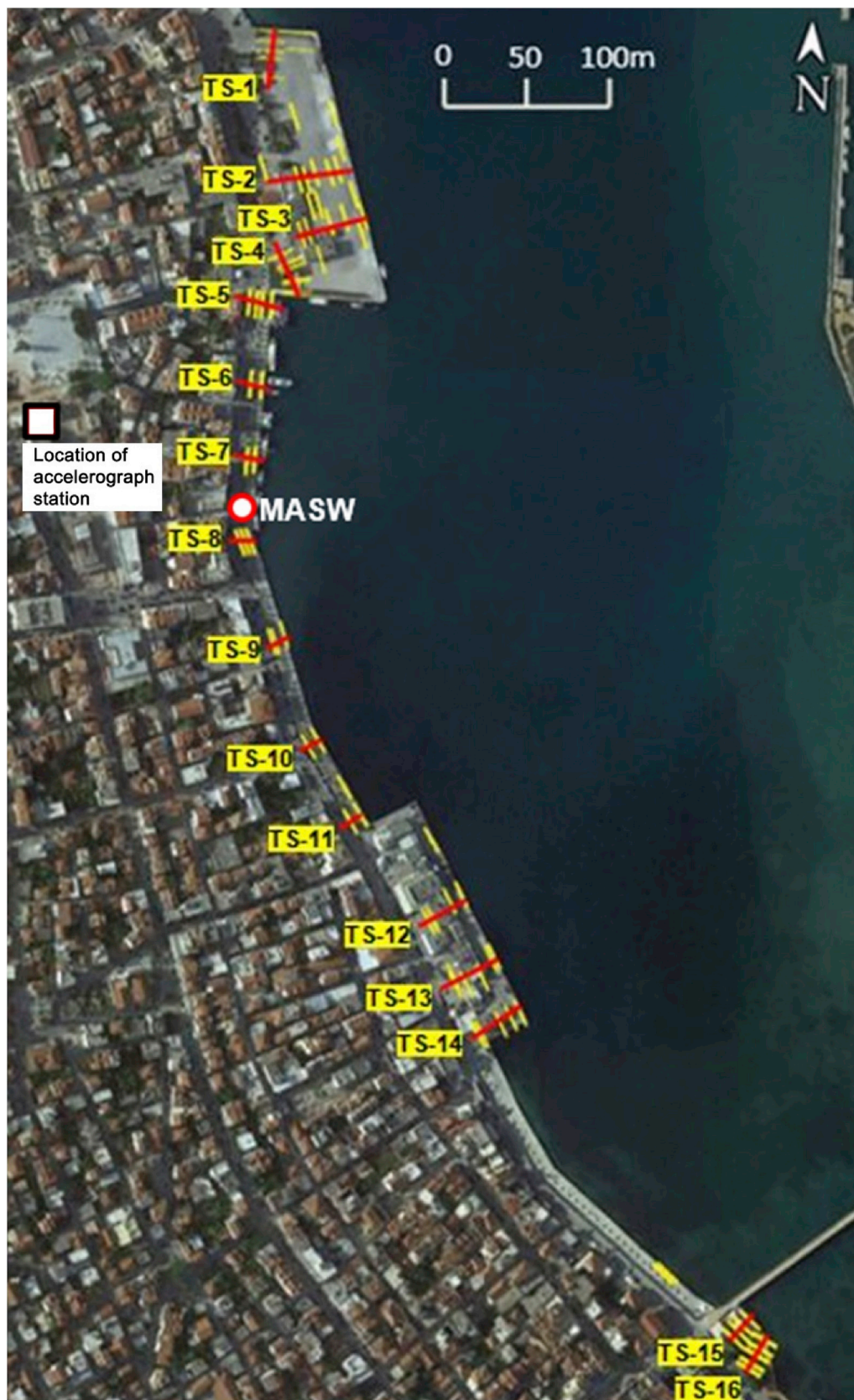
Fig. 7. Location of the sixteen transects surveyed in the Argostoli Port area (with corresponding crack positions), and the accelerograph station which recorded the 2nd event.
