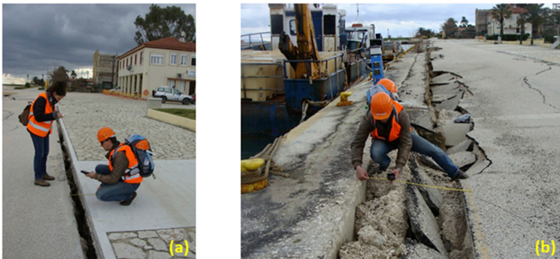
Fig. 5. Field measurements of crack widths due to liquefaction-induced lateral spreading in the Cephalonia 2014 earthquakes.
