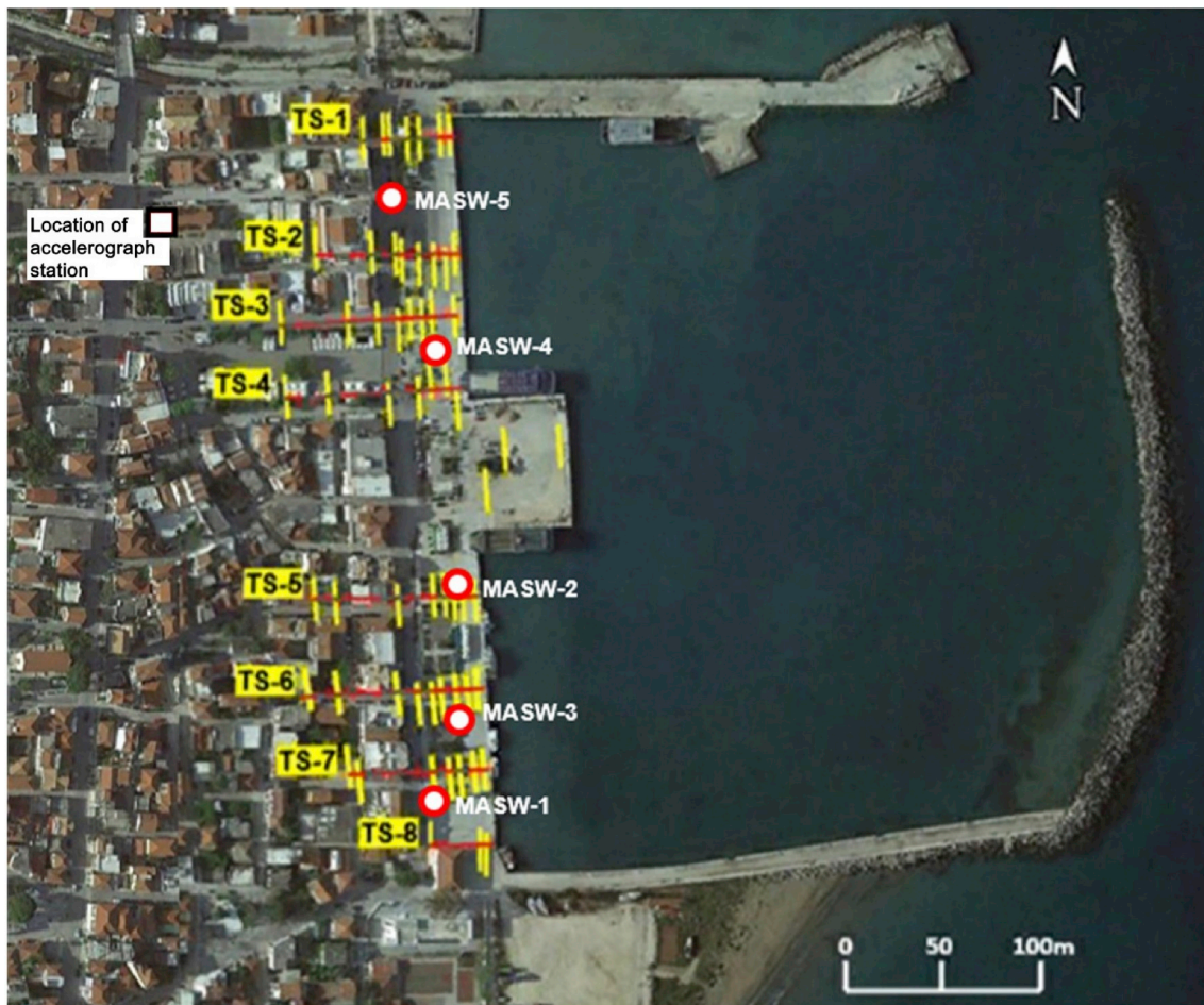
Fig. 6. Location of eight transects surveyed in the Lixouri Port area (with corresponding crack positions), and the accelerograph station which recorded the 2nd event.
