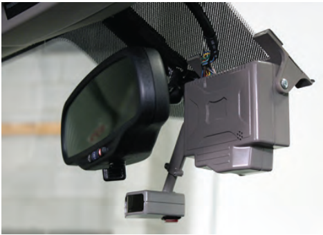
Fig. 1.a. A head unit of the DAS recording four camera views
