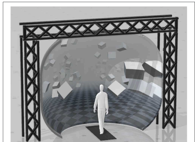
FIGURE 1 | Experimental setup displaying the position of the split-belt treadmill in front of the curved screen.
