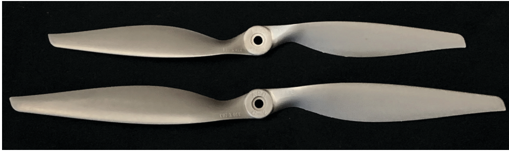
Figure 8: A photo of the two propellers tested: APC 11×10 E (top) and APC 13×8 E (bottom)
