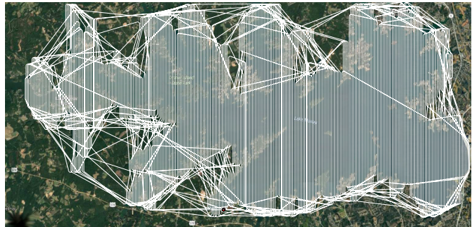
Fig. 1. A path by our planner covering a lake in a search-and-rescue simulation.
