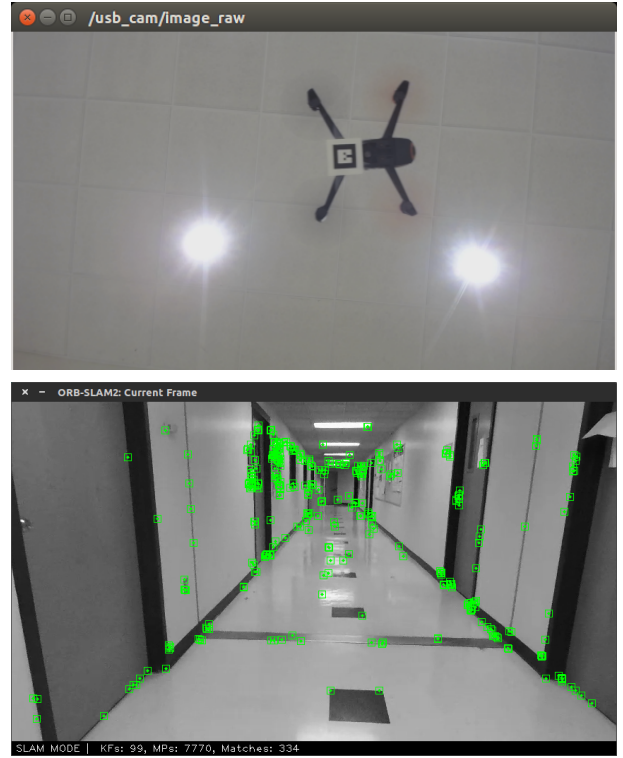
Fig. 5. Camera feeds: In the top image, the Bebop 2 flies over the UGV with a tag. The bottom image shows the UAV's front camera view.
