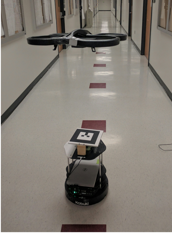
Fig. 4. Early approach using a Parrot AR.Drone 2.0 and the tag on the UGV.
