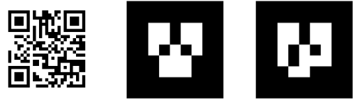
Fig. 2. An example of a QR code is shown first, while two fiducial tags generated by ar_track_alvar are shown after.
