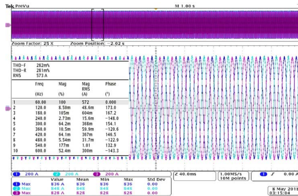
Fig. 9. Current at the PCC (grid-tied mode).
