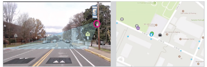
Figure 9. An infrastructure camera captures video from its field of view (left) and the information is displayed in real-time on the mapping application (right).
