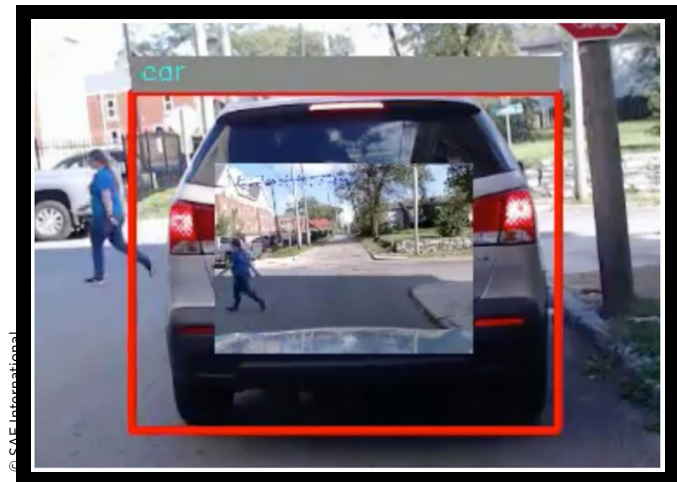
FIGURE 13 A pedestrian exiting the view of the front vehicle and the see-through algorithm's field of view from the front vehicle and into the rear vehicle's field of view.
