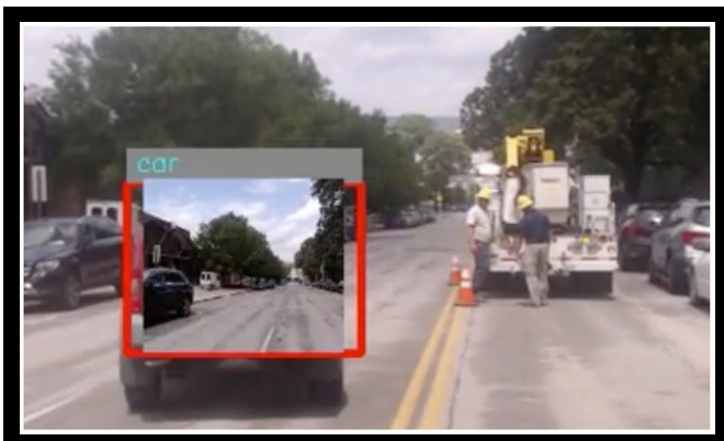
FIGURE 9 A screenshot showing the electric company's truck entering the full view of the rear vehicle's line of sight. This image also shows the driver of the rear vehicle the lane to pass the truck is clear of vehicles driving in the opposite direction and they can follow the vehicle in front to safely avoid the electrical truck as well as the workers.
