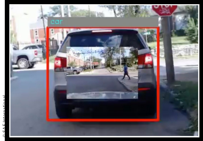
FIGURE 12 A pedestrian crossing the street being viewed by the rear vehicle via the see-through algorithm
