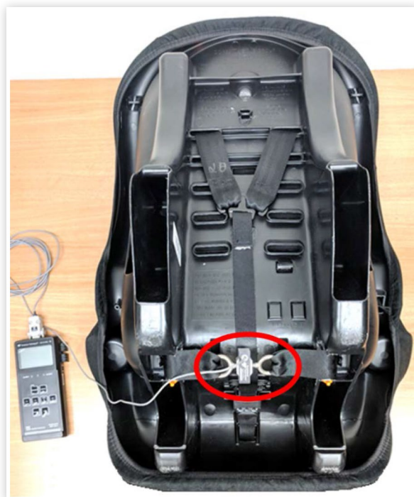
FIGURE 1 The load cell was incorporated into the webbing system underneath the seating surface of the CRS.
