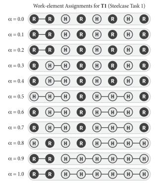
Fig. 6. Work-element allocations for human (H) and robot (R) workers for T1 under different values of  $\alpha$ .
