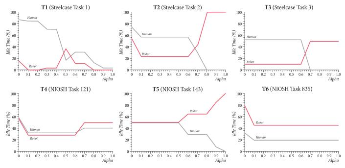
Fig. 7. Idle times for the human (gray) and robot (red) workers for each task. Idle time allows the human worker to recover from fatigue. Based on the physical demands of the task, an acceptable idle time for the human worker may vary. Similarly, idle time of the robot may provide it with opportunities to multitask.
