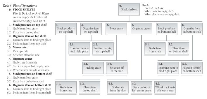
Fig. 4. HTA model of T4 presented in numbered-list and hierarchical-diagram formats based on standard conventions of HTA modeling [29], [34]. In the task, a worker restocks the pantry of a commercial kitchen one crate at a time. The full HTA model, in addition to the goals, tasks, and operations shown earlier, includes task parameters, such as the number of repetitions, duration, and cycle time.
