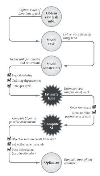
Fig. 2. High-level summary of the process followed by our approach. Capture video showing several iterations of a task. Break down tasks to work elements using HTA through a manual analysis of the videos. Given the work elements, model task parameters, and constraints from video. Estimate times for each work element as completed by the robot. Compute SI for each possible work-element assignment. Send the data to the optimizer.
