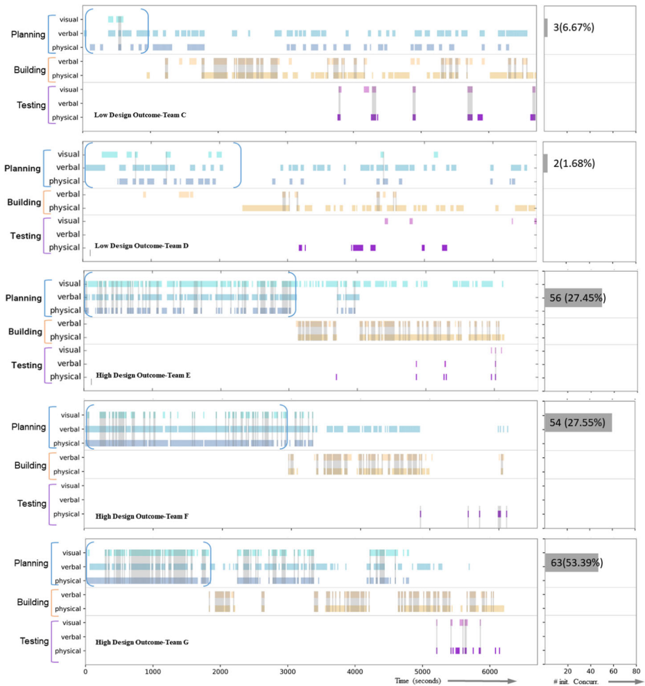
Fig. 4 Design stages and modalities of the low (Teams C and D) and high (Teams E, F, and G) design outcome teams in the trebuchet activity. The colored lines represent the design modalities in the different design stages coded at 15 s intervals. The square brackets indicate the initial phase of the planning stage. The vertical light-gray lines highlight the concurrence of verbal, visual, and physical modalities in the initial planning stage. The horizontal gray bars on the right represent the total number of the concurrent use of the modalities in the initial phase of the planning stage
