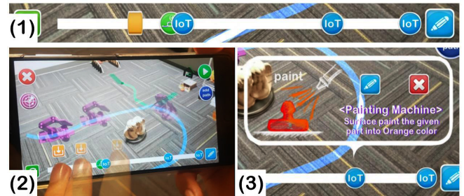
Figure 7. (1) EventLine represents the task in a linear and compact format. (2) User can drag the handlebar to preview with a virtual robot. (3) User can tap on the icon to review its detailed information, and to edit or delete it.
