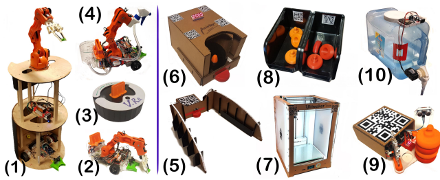
Figure 11. Prototyped robots and IoTs. (1) TowerBot (2) GripperBot (3) SweeperBot (4) WaterBot (5) Charging Station (6) Painting Machine (7) 3D printer (8) Sorting Box (9) Storage Station (10) Water Station
