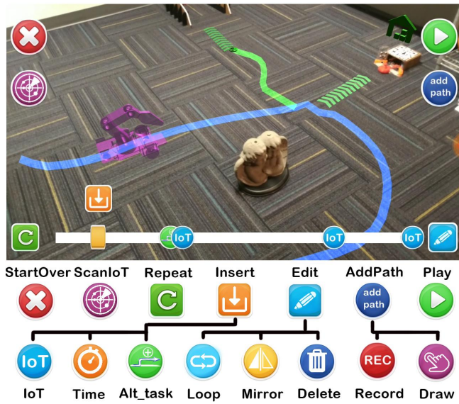
Figure 4. Main interface design of V.Ra system (top). An icon reference list for interactive functions in the system (bottom).
