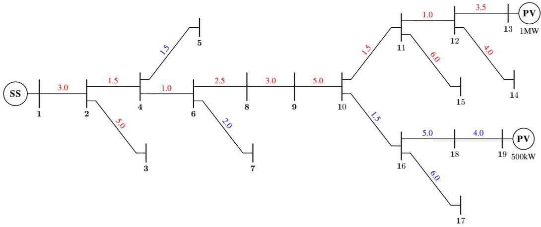
Fig. 1. Single line diagram of the 19-node system
