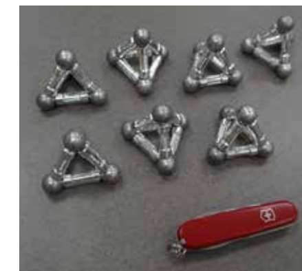
Fig. 5: Arrangement of steel balls and magnetic rods into tetrahedra in the arrangement of Isolated Tetrahedron Silicates (Olivine)
