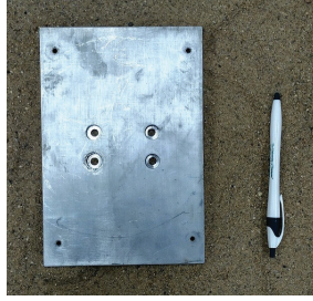
Fig. 12. Aluminum plate used as a buried target.
