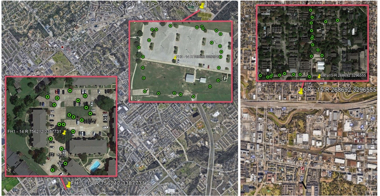
Fig. 5. The ground truth locations in the UTM coordinate system of two fire hydrants in College Station, TX and a tower crane in Houston, TX (FH: fire hydrant, CR: tower crane). The enlarged regions display the data collection areas and the green dots represents the data sample locations.
