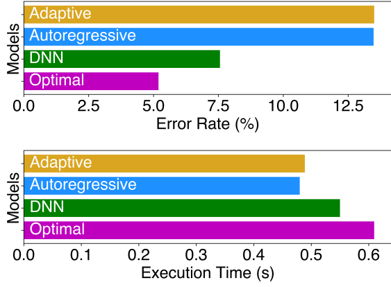
Fig. 4. Comparison of sampling algorithms with sub-second data collection frequency
