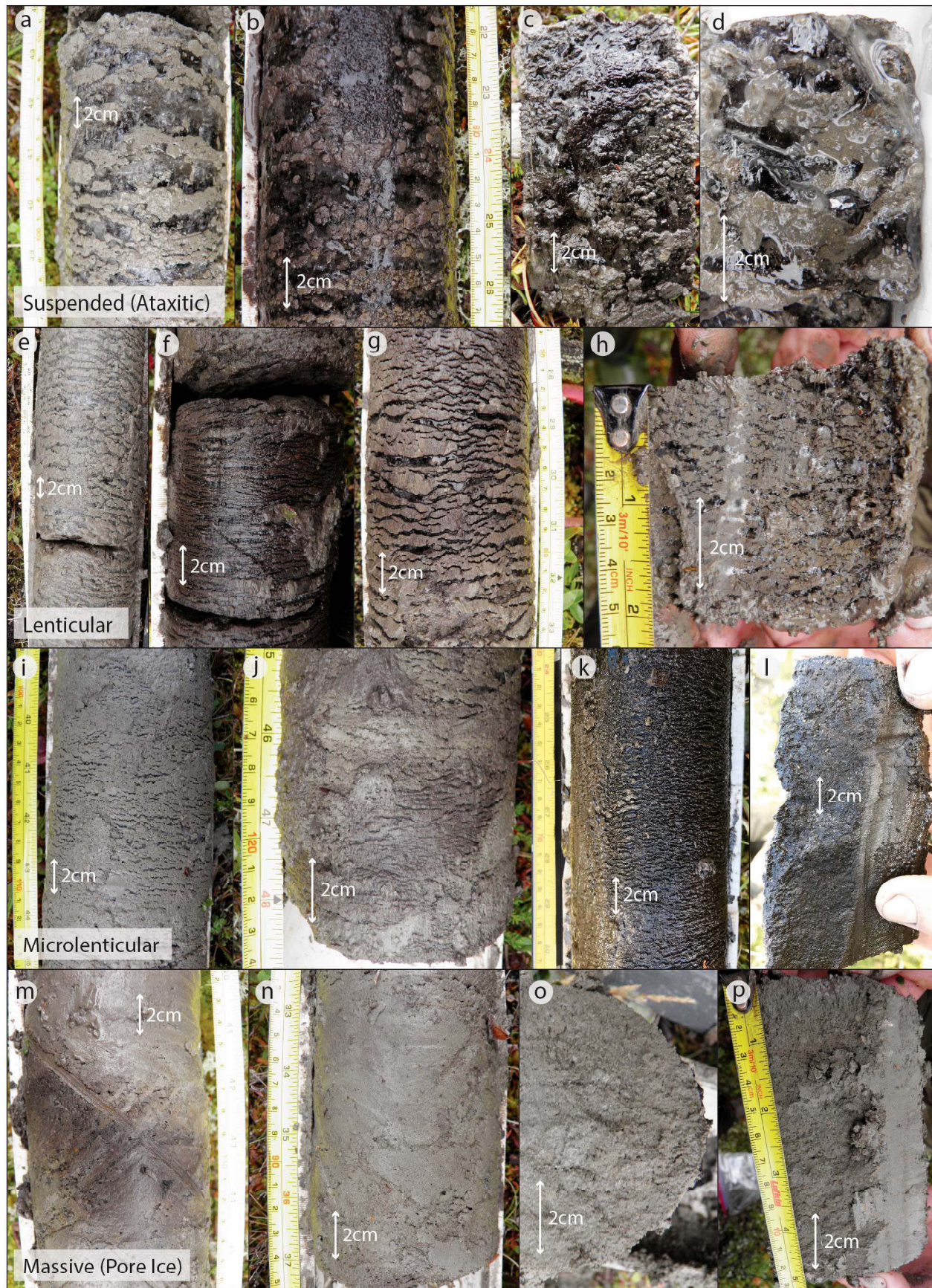
Fig. 5. Typical cryostructures observed in near-surface permafrost under late-successional black spruce in the Copper River Basin, AK. (a–d) Suspended (ataxitic); (e–h) lenticular; (i–l) microlenticular; (m–p) massive (pore ice).
