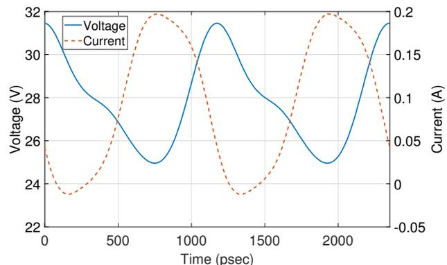
Fig. 3. Small-signal intrinsic drain voltage and current waveforms showing a significant second harmonic component.
