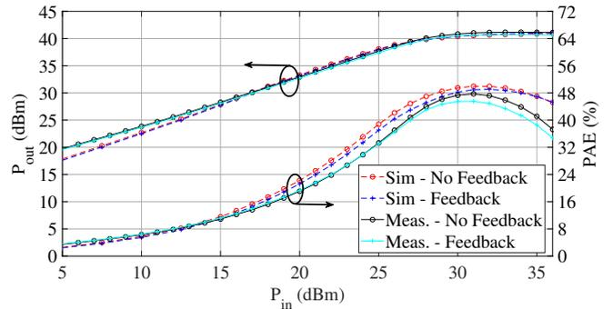
Fig. 5. Simulated and measured CW output power and PAE of PA with and without IF feedback at 5MHz present.
