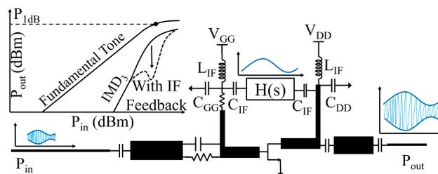
Fig. 1. Block diagram layout of a power amplifier capable of suppressing intermodulation distortion under a high input power, complex modulation excitation through IF feedback.
