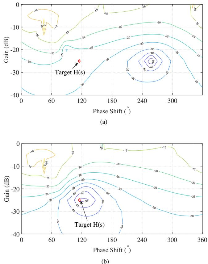
Fig. 2. Simulated (a) upper and (b) lower IMD3 under 5-MHz spaced tones with 24-dBm input tone power as a function of baseband feedback transfer function at 5 MHz.
