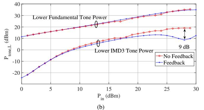
Fig. 6. Measured fundamental and IMD3 tone power under 5 MHz tone spacing for (a) upper and (b) lower tones compared with and without feedback.
