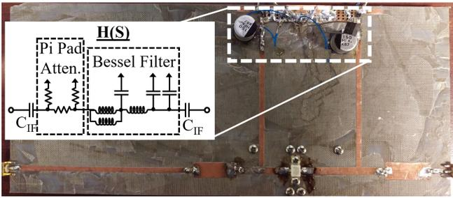
Fig. 4. The 215.9 mm by 88.9 mm baseband feedback power amplifier.
