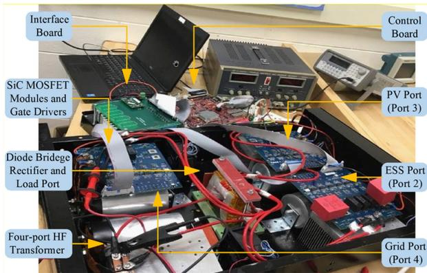
Fig. 10. Implemented 10 kW/port MPSST in the lab.
