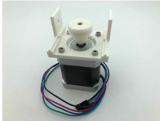
Fig. 5. Motor_mount_top and the shaft coupler attached to motor using M3x8 bolts.
