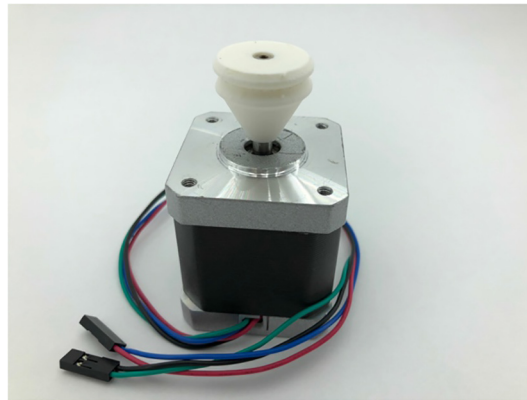
Fig. 4. 3D printed shaft coupler (white piece) mounted on the motor.
