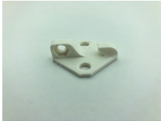
Fig. 13. Line_Tie2 3D printed piece that will have the fiber attached to it.
