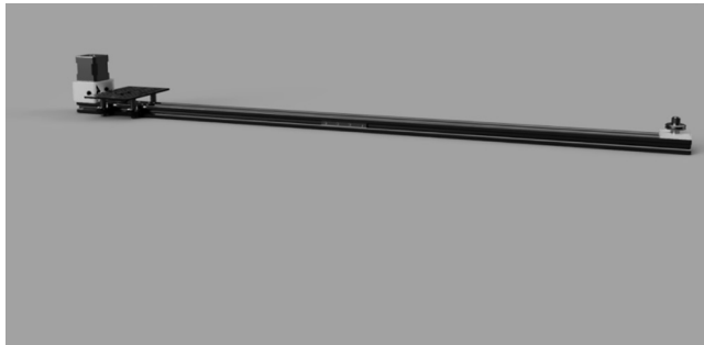
Fig. 26. CAD assembly of 1-meter HyperRail demonstrating the assembly of the carriage, motor, and idling pulley.
