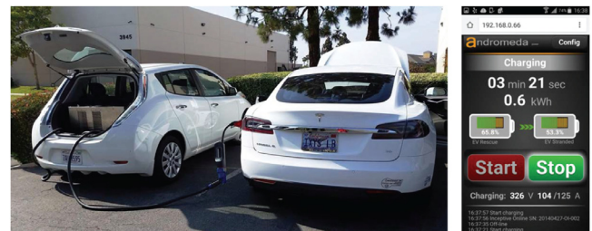
Fig. 6. Infrastructure-free case: Electric vehicles can exchange energy anywhere through a DC/DC converter and a conductive charging cable. A mobile app communicates with both vehicles and lets the drivers control the charging process [35,141].
