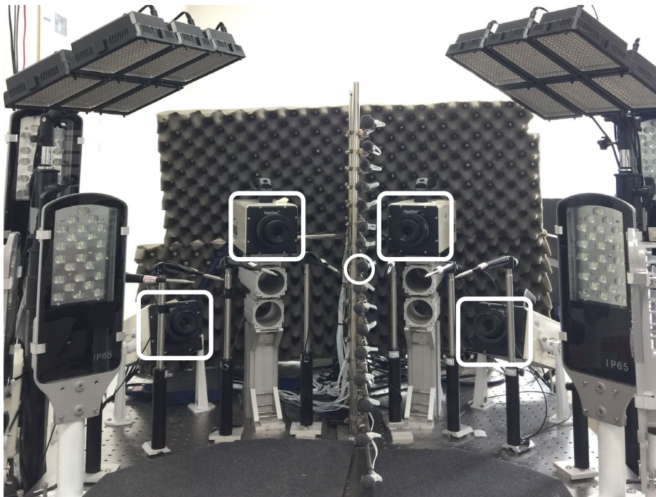
Fig. 2. Experimental setup. Four high-speed video cameras (marked by white squares) were used to record the three motion trajectories of the landmarks on the noseleaf and pinnae. An ultrasonic measurement microphone (white circle) was used to record the bats' ultrasonic pulses. Recordings from the cameras and the microphone were triggered simultaneously. Illumination was provided by six sets of LED lights (seen in the two upper image corners).
