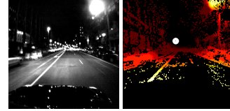
Figure 7: Failure case of our depth network. The flashing street light is detected as very close due to spurious events.
