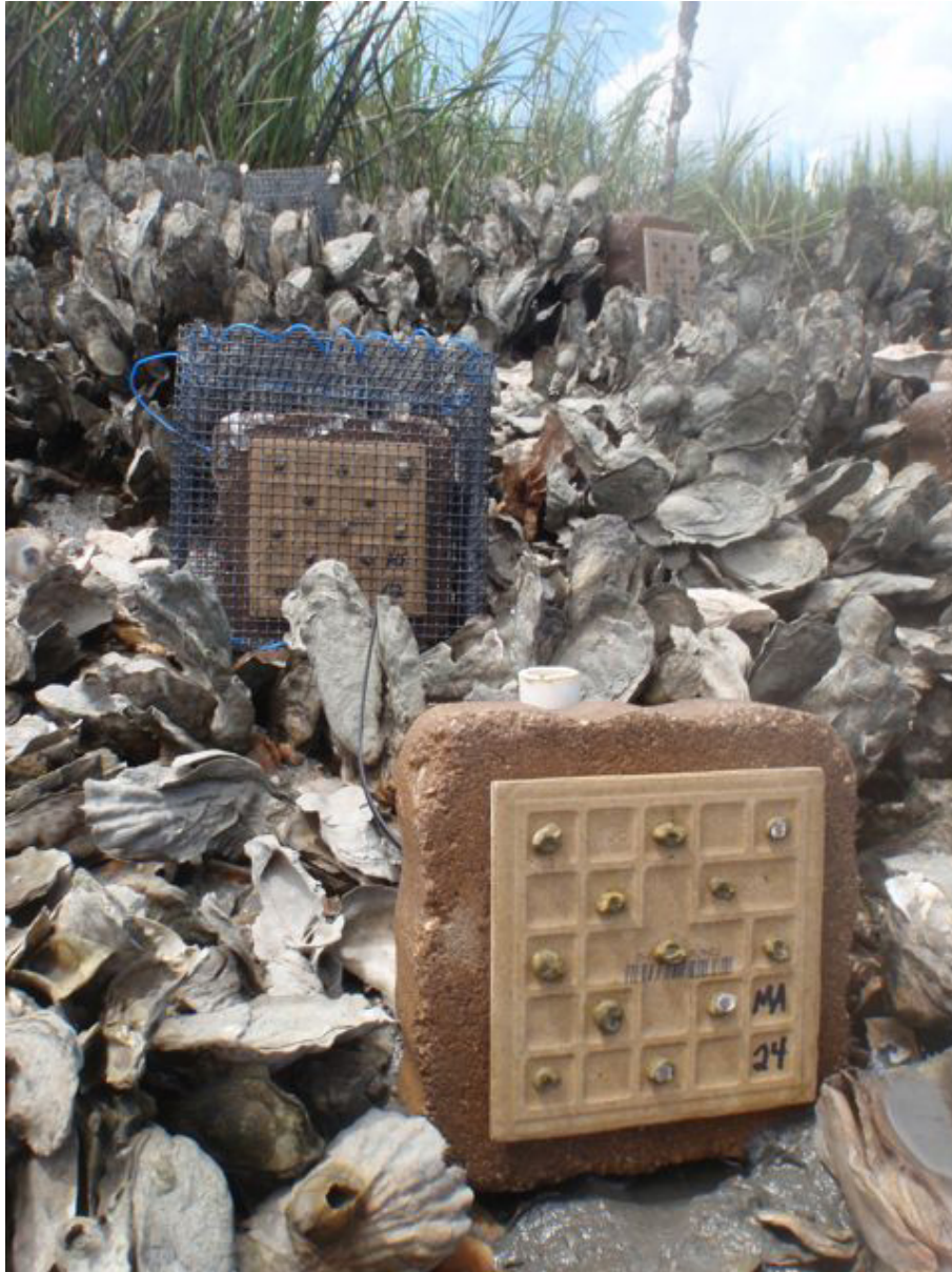
Photo 2. Identifying the role of predators in oyster mortality. Tiles were caged (background) or uncaged (foreground) to test the effects of predation. Photo credit: J. Byers.
