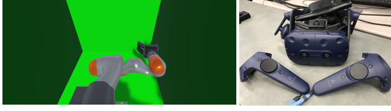
Figure E.1: VR setup. Left: VR environment as viewed from the Vive headset. The green box represents the position constraints on the end effector. The end effector is commanded to move by dragging it with the HTC Vive controllers ( right ).
