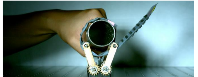
Fig. 1. A visual illustration of our bi-stable gripper design closing when activated with by a mechanical collision with a tube.
