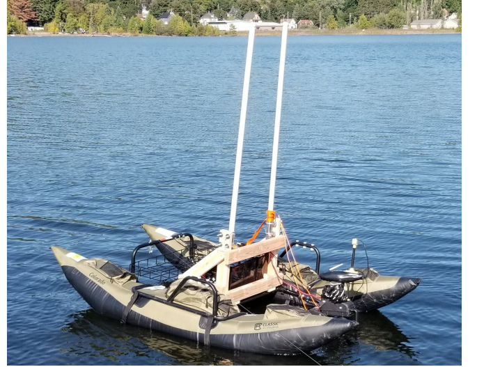
Fig. 7. Image of an autonomous surface vehicle developed for establishing an underwater communication infrastructure.
