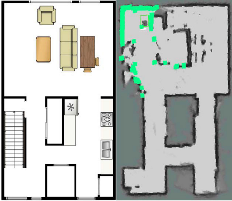
Fig. 7. Actual layout for bottom floor of smart home with added furniture from Figure 2 (left) and RAS-learned map of navigable smart home regions (right). In the robot map, green dots highlight the current LiDAR scan and the dark green rectangle represents the robot's bounding box.
