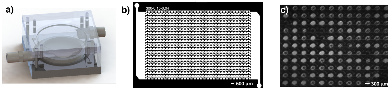
Figure 2. (a) The design of the cold plate assembly with the microfluidic chip enclosed in an acrylic chamber. (b) Top view of the darkfield mask used to fabricate the microfluidic device master mold, showing the array of 720 individual microwells. The device has 24 parallel channels along each row and 30 equally spaced microwells per row. (c) Top view of the droplet-filled device placed on a gold-coated silicon wafer during a cooling assay. The gold-coated silicon wafer acts as a mirror and a double image can be seen for the liquid droplets (clear/dark) and frozen droplets (white).
