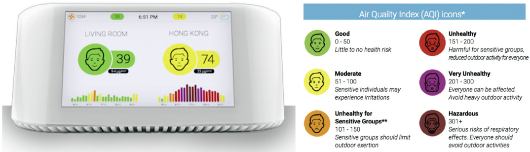
Fig. 3. AirVisual, an IAQ monitoring station that uses colors, graphs, numbers, and icons to visualize IAQ (left) and the AQI icons with different facial expressions (right).. (For interpretation of the references to color in this figure legend, the reader is referred to the web version of this article.)
