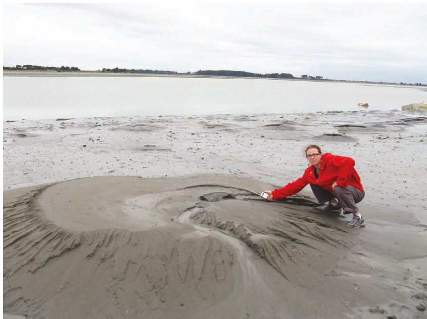
Figure 5. Severe surficial liquefaction manifestations in the Avon-Heathcote Estuary that formed during the 2011 M 6.2 Christchurch earthquake, where the PGA at this site estimated to be greater than 0.6 g (photo courtesy of Greg DePascale, February 22, 2011).
