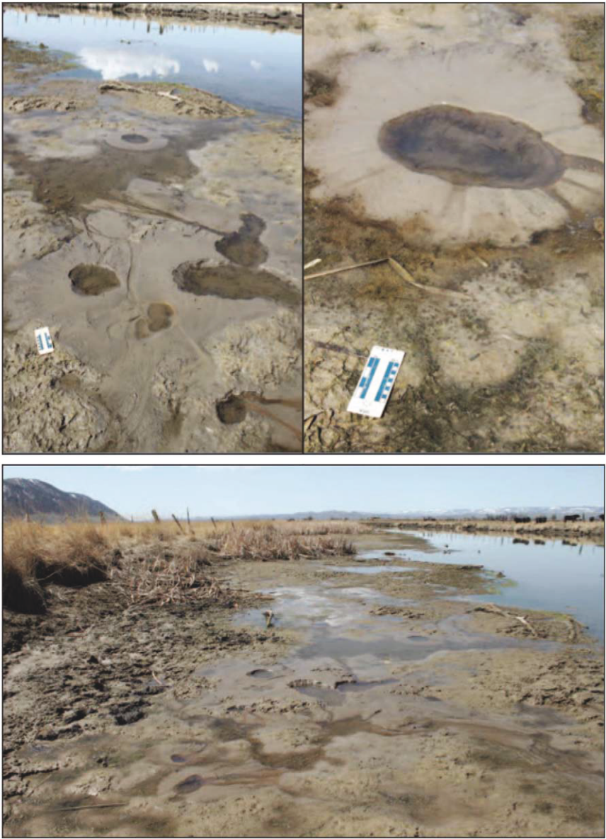
Figure 2. Liquefaction effects observed following the M 4.6 Randolph earthquake in Utah (Pankow et al. 2015).
