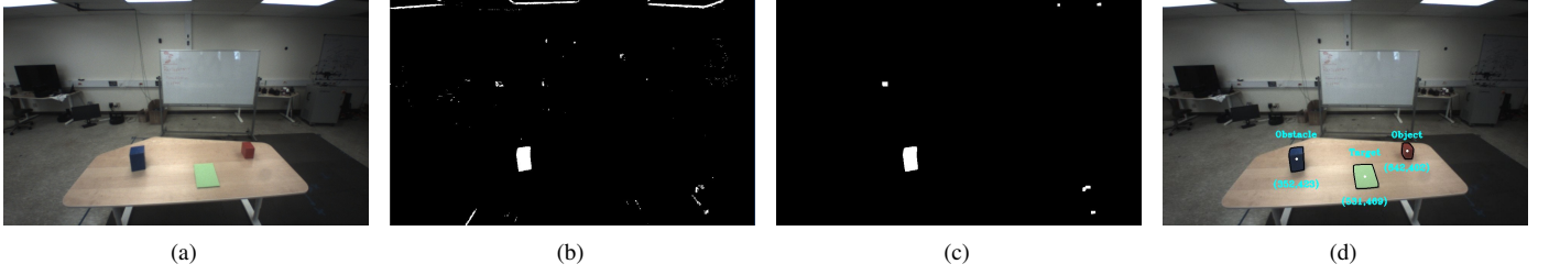
FIGURE 4. HSV-based scanning for object detection: (a) Original image; (b) Binary mask of "Blue" pixels; (c) Mask after morphological filtering; (d) Image with contours and centers drawn
