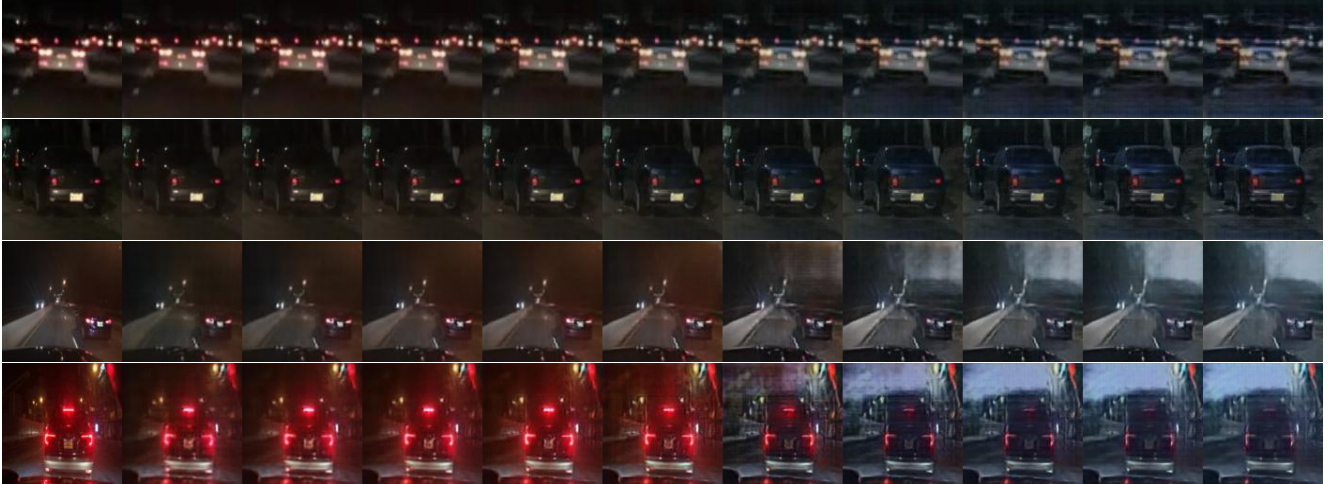
Figure 4. Style manipulation of time of day attributes through a trained Attribute GAN with day and night labels. The first column shows the original image. The next ten columns denote the gradual change in style which is the time of day in this case. The first two rows show gradual change from night to day on images from the test set of crop images. The last two rows exhibit gradual change from night to day on images from the original BDD dataset. This shows that the model trained on crop images from the original dataset generalizes on the original uncropped BDD images. Note that the model learns intuitive transformations by dimming taillights or clearing the sky.
