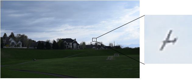
Fig. 8. Flight testing image (left) and cropped image (right). The crop is sent to the CNN to create a measurement. The original image was 1920 \times 1080 and the crop is 50 \times 50 pixels.
