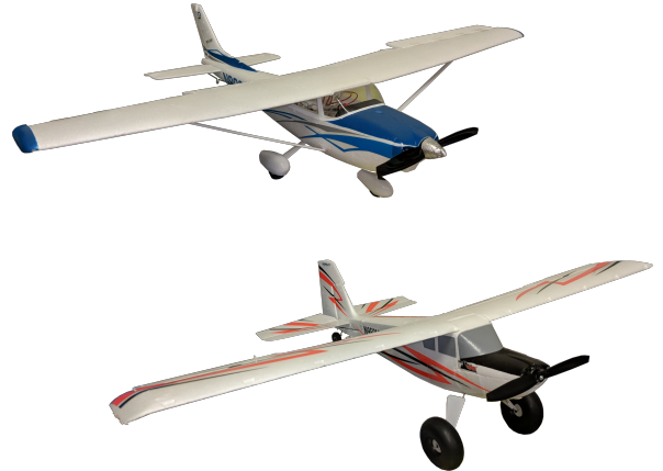
Fig. 1. This paper will demonstrate a feasible method for estimating the state of an RC aircraft, such as these, using deep learning and only third-person-perspective visual sensing. This UMX Cessna 182 and UMX Timber by Horizon Hobby were selected for testing the proposed method because they are visually representative of the high-wing airplanes used to train the CNN.
