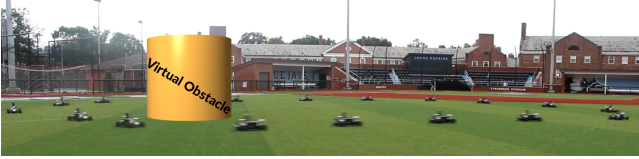
Fig. 3. The robot using an optimized control policy to follow a 22 m \times 14 m oval track at 6.5 m/s while avoiding virtual obstacles.
