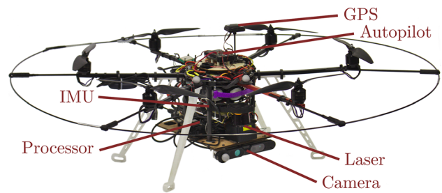
Fig. 11 The vehicle used for the flight tests
