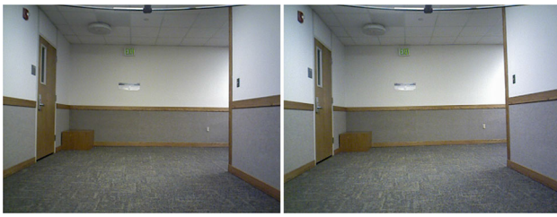
Fig. 8 Example loop closure detected using FAB-MAP between keyframe 80 and keyframe 416 during flight test 2
