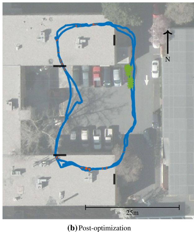
Fig. 19 Pose-graph map for flight test 3. a Trajectory (blue) before incorporating loop closures (red) and GPS measurements (green). For plotting purposes, the GPS is plotted relative to the first received GPS measurement. b After incorporating the ten available GPS measurements (green), the trajectory is globally localized. Black indicates the doorways. Note that because all of the available GPS measurements were slightly biased to the north, the final map is also biased (Color figure online)
