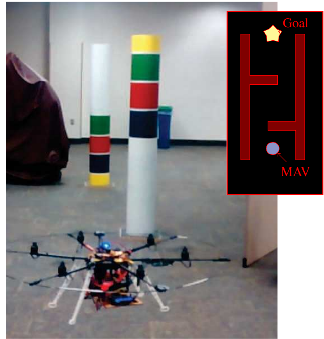
Fig. 8. Hardware validation of CEPA in a GPS-denied environment using strictly onboard computation and sensing.
