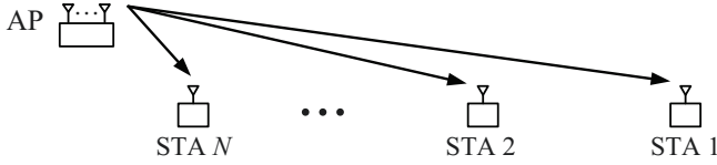
Fig. 1: Downlink data transmission in a WLAN.
