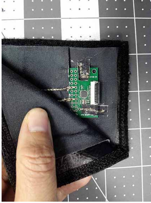
Figure 5: Conductive threads connected to ground, shield and capacitive sensors connect to Capsense daughter board in the RestEaZe band.
