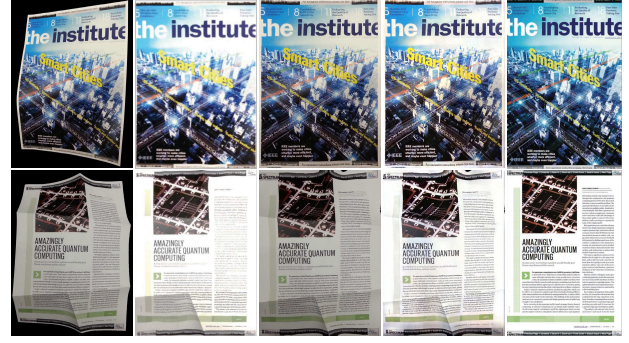
Figure 8. Comparison with You et. al. [45]. Columns from left to right: 1) Original warped images, 2) Results from [45], 3) DewarpNet, 4) DewarpNet results after shading removal, 5) Flatbed scanned images.
