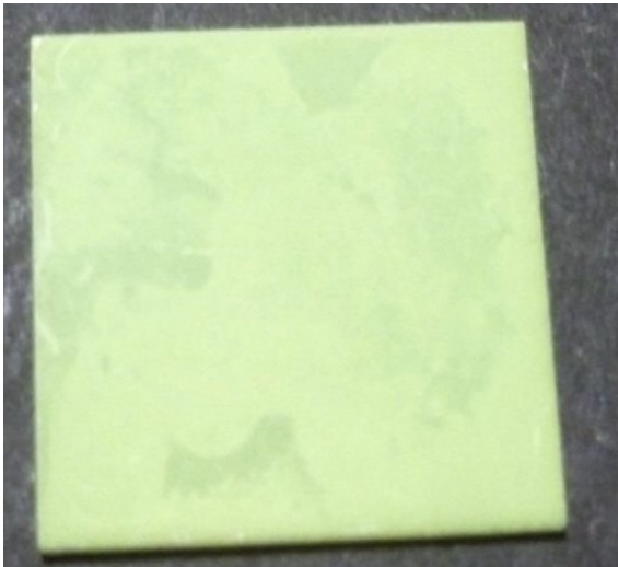
Fig. 7. 2cm x 2cm x 1 mm (5 micron) Incom/bismuth polymer. A 2cm x 2cm plate has more than 20,000,000 capillaries.
