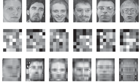
Fig. 5: Example images and their corresponding obfuscation. Row 1 - original AT&T images ; Row 2 - images in Row 1 obfuscated by Pix-DP [7] for each 16 \times 16 -pixel grid cell with \epsilon = 0.3 ; Row 3 - images in Row 1 obfuscated by our method SVD-priv with k = 4 and \epsilon = 0.3 .
