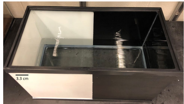
Fig. 2 Aerial view of the custom-built scototaxis testing chamber. Frogs were given 10 min to acclimate within an opaque tube in the center and were then allowed to swim freely during testing
