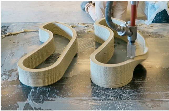
Fig. 9. Elastic buckling during a 3D printing process.
